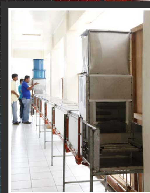
The pilot-scale unit dryer is tunnel shaped and made of food grade stainless steel.
